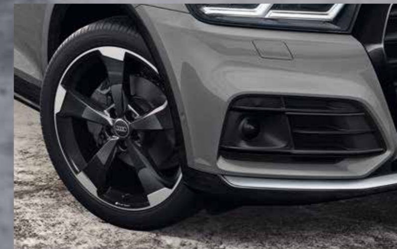
Bottom front bumper section with aluminium clip – 20-inch Audi Sport cast aluminium wheels in 5-arm rotor design in gloss anthracite black, gloss turned finish 1, 2
