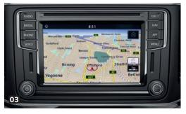
Discover Media navigation system. In addition to the functions of the Composition Media radio system with six loud speakers, there is a second integrated SD-card slot which is compatible with the SD-card with the map data. |HL|UL|HLB|
