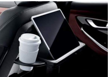
Front row seatback table with retractable cup-holder and IT device holder
