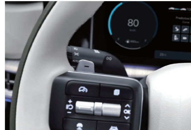
Hybrid Exclusive Features Paddle Shift-Regenerative Braking Mode
