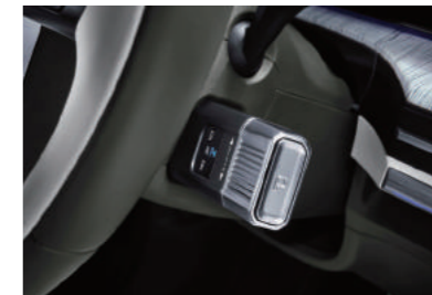
Column-type Shift by Wire (SBW)
