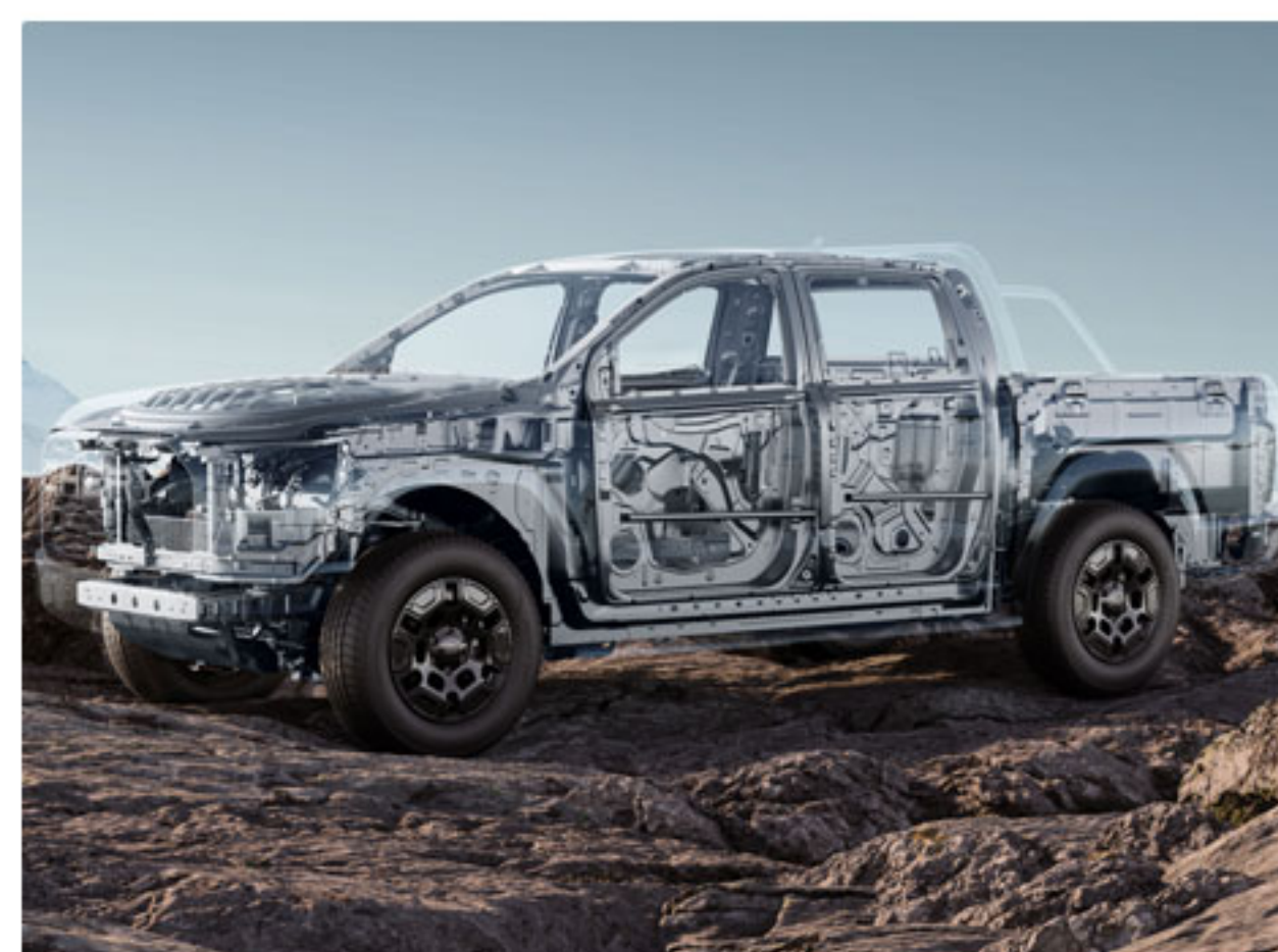
High-Strength Body with Galvanized Steel Plate & Anti-collision Steel Beam
