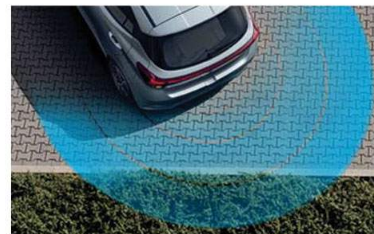
Rear Parking Assist System
